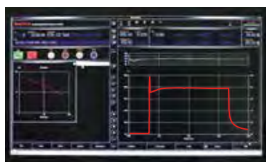
Mooney Viscosity test with stress relaxation and log-log graph
