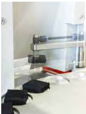
Sample queueing and sample detection sensors for fully monitored sample handling.
